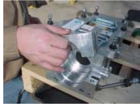
Figure 2 Remove Duct Clamps
