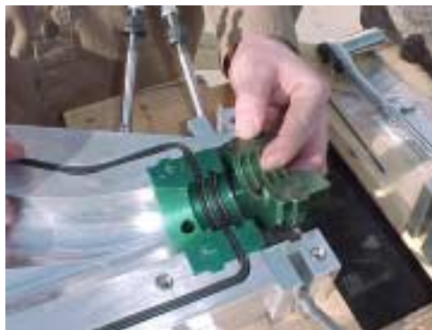
Figure 4 Inseart Duct Clamps
